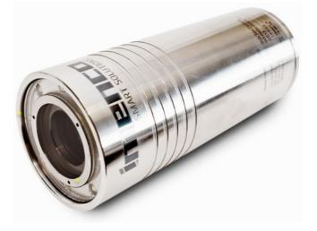
The Imenco Whitetip Shark II<sub>IP</sub> Colour Zoom Camera incorporates a Sony STARVISTM CMOS sensor and features a 10x optical zoom lens. With built-in LED lights and ultra-compact and a lightweight Titanium housing rated to 4.000msw, it is an ideal camera for inspection of restricted spaces and in tooling applications.
