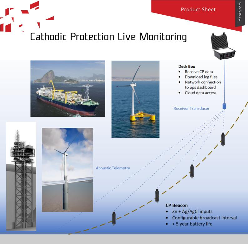
With an extensive track record of acoustic communication, Imenco provides long term wireless live monitoring of level of protection of installed Cathodic Protection (CP).
