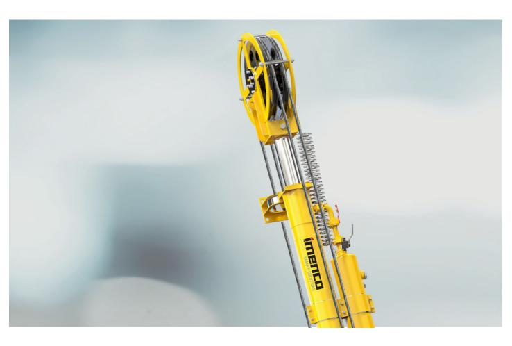
GLT Is a hydro pneumatic device used on an offshore drilling rig or vessel It keeps a constant positive pulling force on the guide wires from the rig to a template on the seabed. The guide wires act as guidance for equipment and tools that must be lowered to the template. Without a tensioner, the guide wires would become slack and could be broken if the platform moved. In recent years we have developed several types of wire tensioning systems.
