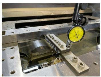
Electrical Discharge Machining is a controlled metal-removal process Electrical Discharge Machining (EDM) is a controlled metalremoval process that is used to remove metal by means of electric spark erosion. In this process an electric spark is used as the cutting tool to cut (erode) the workpiece to produce the finished part to the desired shape.
