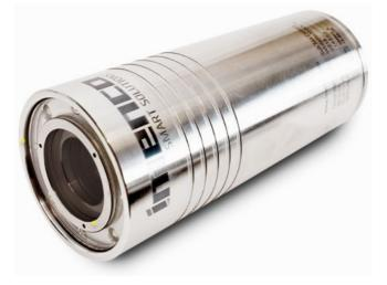
The Imenco Whitetip Shark II<sub>HD-SDI</sub> Colour Zoom Camera incorporates a 4Mpx - 1/3" CMOS sensor and features a 10x optical zoom lens. With built-in LED lights and ultra-compact and a lightweight Titanium housing rated to 4.000msw, it is an ideal camera for inspection of restricted spaces and in tooling applications.
