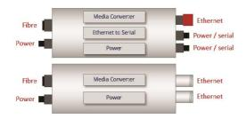
The Imenco ICON Mux makes use of one spare fibre / wave length, in the existing ROV mux / umbilical for transmission of full HD IP video and serial signals for LED lights and P/T control.
