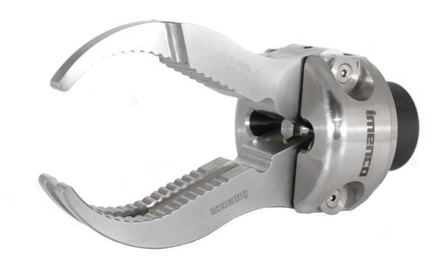
There are over 300 Imenco jaws at work Globally The 3 & 4 fingered manipulator jaw is intended as a hydraulically operated tool. The front adapter assembly comes complete with actuation plate and piston and all necessary gaskets and will replace the standard parallel grip by loosening the 6 bolts.
